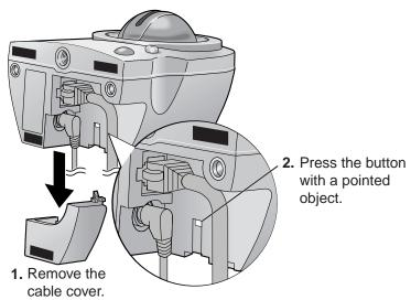
Pressing the FACTORY DEFAULT RESET button resets the camera to factory default. If you lose your user name and password, use this button to reset the camera.
